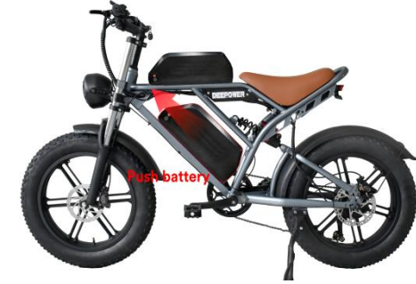
03 After unlocking the battery, push the battery upward to remove it (you need a lot of force because the battery is heavy)
