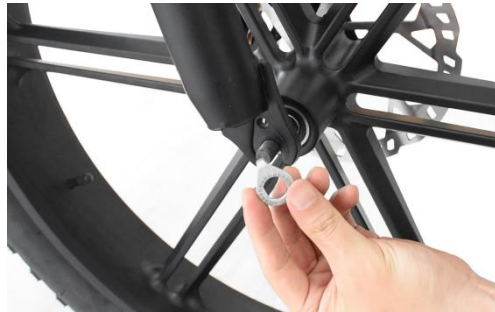
02 Install the part in the shape of the water drop, the upper part of the bend into the hole (very important)
