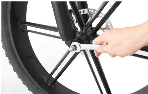
05 Tighten the nut with a wrench
