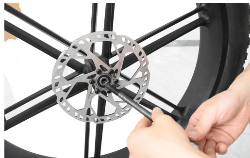
05 Remove one end with a wrench and insert it into the middle of the wheel
