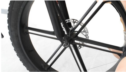
01 Put the wheel on the end of the front fork (you may need help from another person)
