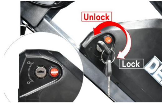
02 The battery is marked with the direction of locking and unlocking
