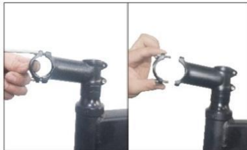
04 Remove front 4 bolts from stem cover them remove stem cover
