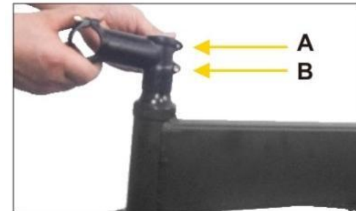
03 Tighten the side A,B screws
